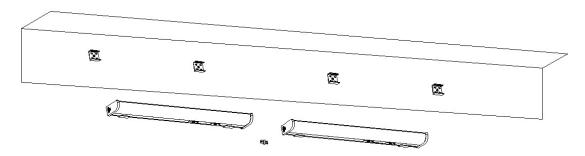
**STEP 3:** Fix the fixtures to the brackets.
