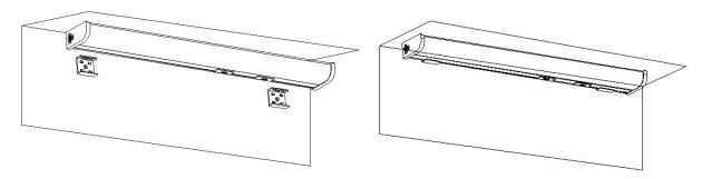
**STEP4:** Plug in the power plug to turn on the fixture.
