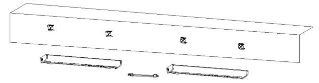
**STEP 3:** Fix the fixtures to the brackets.
