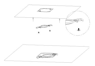
STEP 5 Take out the fixture and connect with male and female fast connector. After ensuring it's firmly connected, tidy the wires and install them on the multifunctional bracket.
