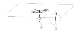
**STEP 2** Fix the multi-functional bracket to the junction box with screws according to the square shown in the figure.
