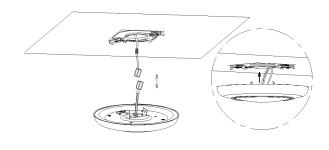
STEP 3 Use a scissor to cut off the E26 adapter, strip the wire to expose the 1CM of copper core.
