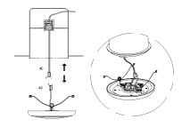
**STEP 7** Press the spring tabs of the fixture and fix it on the bracket of the recessed housing.
