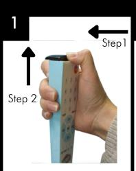
Looking at the keypad, slide the dark lens cover away from you (STEP 1) and lift the lid from the back (STEP 2).
