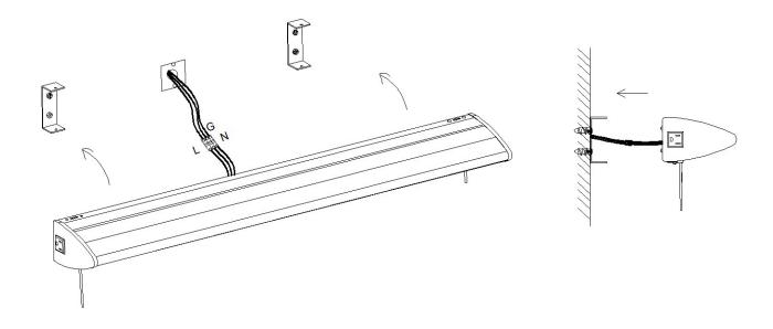
**STEP 4**Fix the light fixture in place with the 4pcs of self tapping screws, each 2pcs for upwards and downwards and make sure it is secure.
