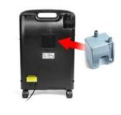
The Stratus 5 HEPA paper filter is located in the back of the unit as shown above. The unit comes with one HEPA filter. This filter should be changed every 10,000 hours and in between patients.
