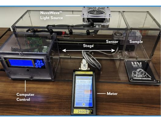
The "Corona Coaster" is our robotic NuvaWave tester that automatically moves the pathogen under the UVC light at a specific rate and has sensors to measure the dose of UVC that the pathogen was exposed to. Also, we can describe our procedure for pathogen reduction using ASTM E3135 standard procedure without soil.
