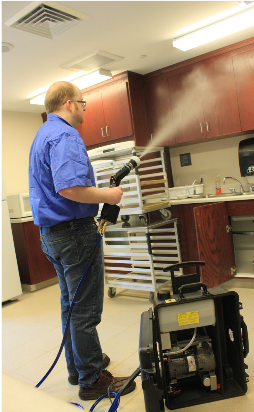
Correct spray technique with similar sprayer, SC-ET-HD
