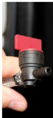
Tank valve closed
