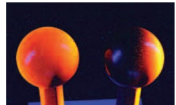
A Picture Worth A Thousand Words... In this test, fluorescent dye has been sprayed on two round knobs. The left knob was sprayed with the electrostatic system ON; the right knob was sprayed with the same sprayer, but with the electrostatic system OFF. Note how even the coverage is on the electrostatic knob.
