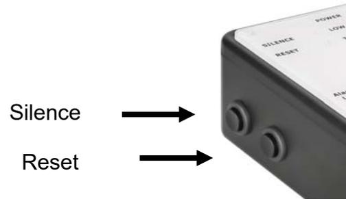
**Silence:** If pressed when any zone is in alarm, Red LED flashing and Audible sounder on, will cause the audible sounder to turn off and the zone Alarm Red LED to change from flashing to steady
