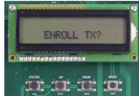
Press "Up" or "Down" to scroll thru the menu for other options or press "BACK" to exit programming mode. Screen will go blank.
