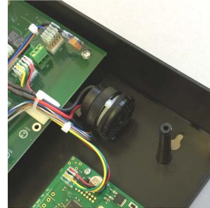
Remove cover and lid to access the internal alarm sounder. Turn baffle on outside of sounder to adjust loudness. Put lid back on bottom and test loudness before re-assembling lid and cover.
