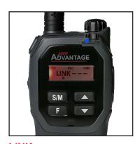
LINK - - - Will be displayed on the screen and the LED will flash blue while connecting.
