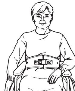
**TO CLOSE AND OPEN THE HOOK-AND-LOOP CLOSURE** Thread “hook” tab through ring on opposite belt section. Bring “hook” over ring and press against “loop” material. To release, simply pull up on hook material.
