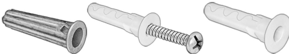
Typical drill size is 5/16" for the #10 conical lead anchor for concrete. Follow manufacturer's instructions. Follow manufacturer's recommendation for drill depth for insert being used.
